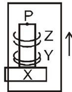
Two ring magnets Y and Z, each of mass  $M$ , are kept in frictionless vertical plastic stand so that they repel each other. Y rests on the base X and Z hangs in air in equilibrium. P is the topmost point of the stand on the common axis of the two rings. The whole system is in a lift that is going up with a constant velocity.
