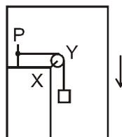
A pulley Y of mass  $m_0$  is fixed to a table through a clamp X. A block of mass  $M$  hangs from a string that goes over the pulley and is fixed at point P of the table. The whole system is kept in a lift that is going down with a constant velocity.
