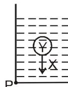
A sphere Y of mass  $M$  is put in a nonviscous liquid X kept in a container at rest. The sphere is released and it moves down in the liquid.
